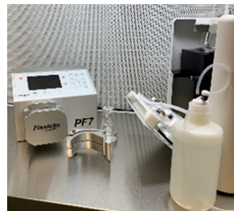
Benchtop filler in Saint-Gobain Life Sciences' lab test environment
